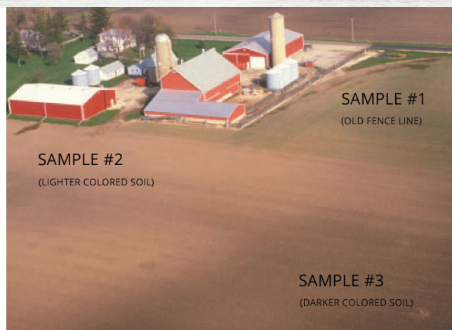
Figure 2. Sampling areas based on variation across the field as indicated by differences in soil type and an old fence line.
