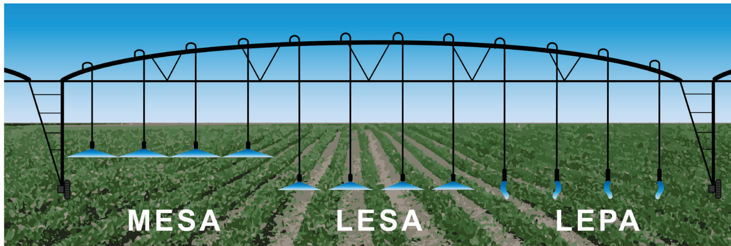
Figure 1. Center pivot layouts; middle-elevation spray application (MESA), low-elevation spray application (LESA), and low-energy precision application (LEPA).
